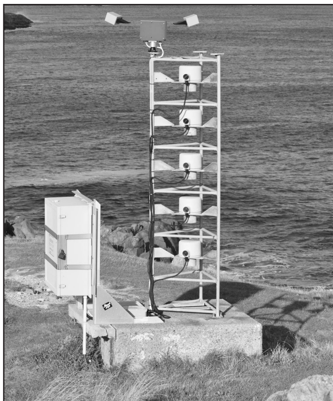
LOUISBOURG'S AB 560 FOG HORN WITH SENTRY FOG DETECTOR MOUNTED ON TOP. CHRIS MILLS
